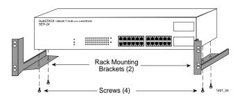
Figure 3-4. Installing the Rack Mount Brackets
